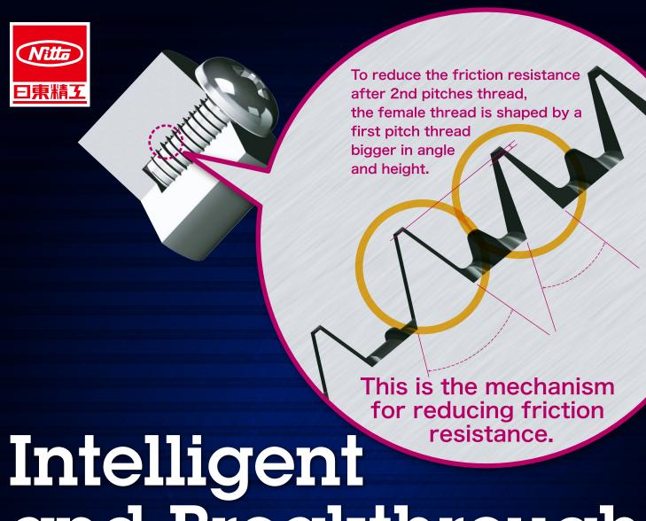
and Breakthrough Prevent adhesive phenomenon when fastening a soft metal workpiece.
